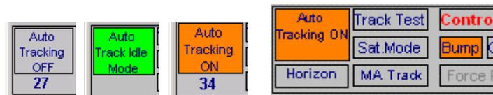
The green label indicates that Auto Tracking is operational but none of the prioritized satellites are above the horizon. The Orange label indicates that Auto Tracking is operational and the satellite with the highest priority is being tracked.
